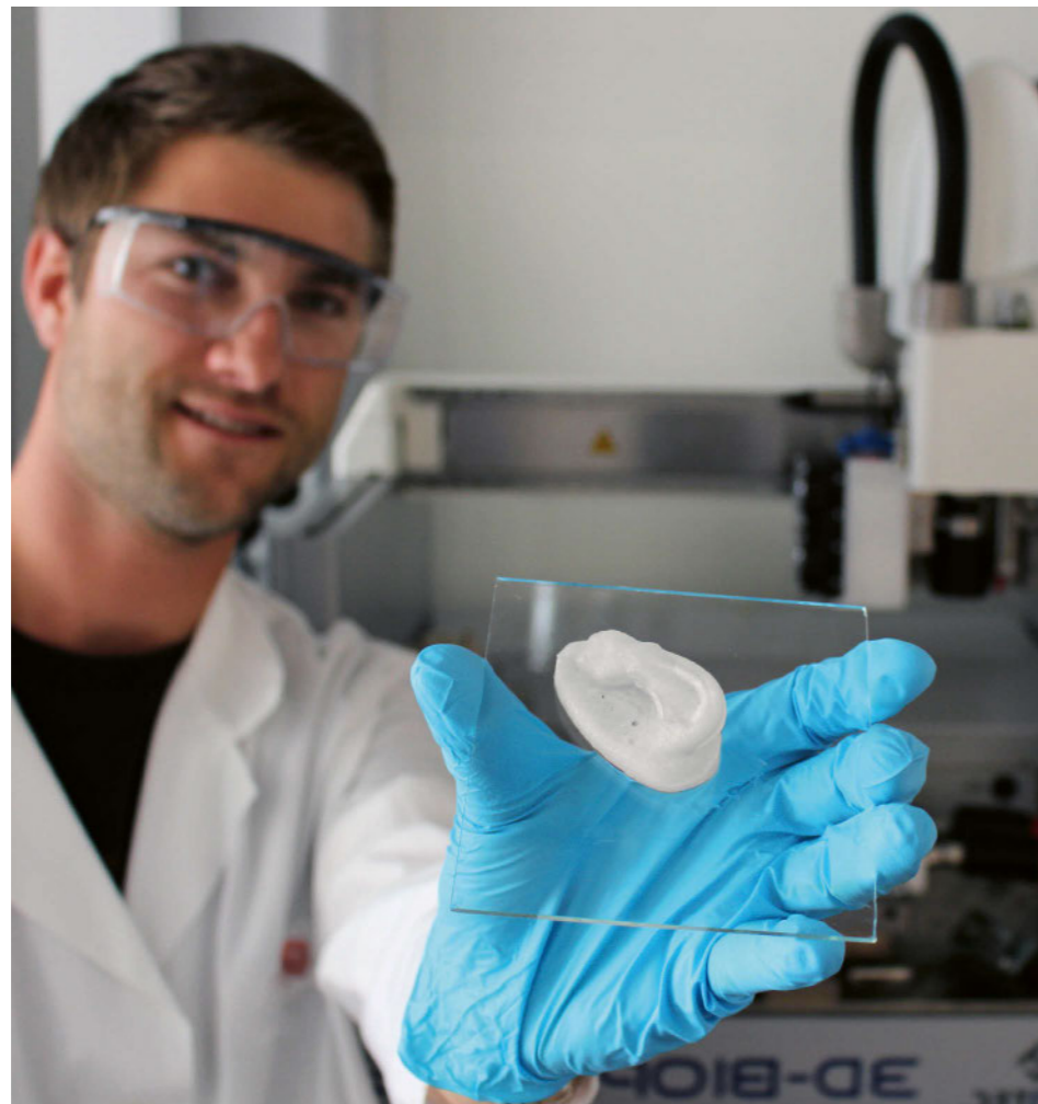
A 3-D- printed ear: Empa researcher Michael Hausmann uses nanocellulose as the basis for novel implants.
