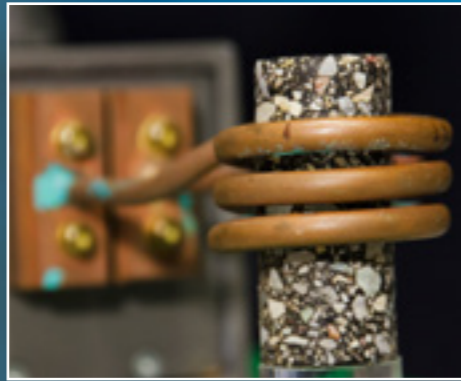
A coil generates a magnetic field around the sample.
