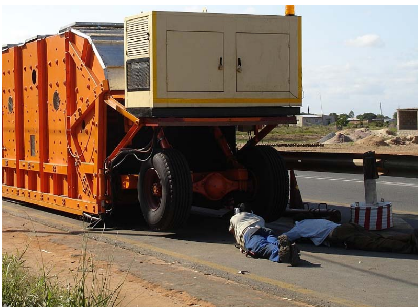
The first tests in Africa: the simulator demonstrating how good it is at destroying road surfaces.
