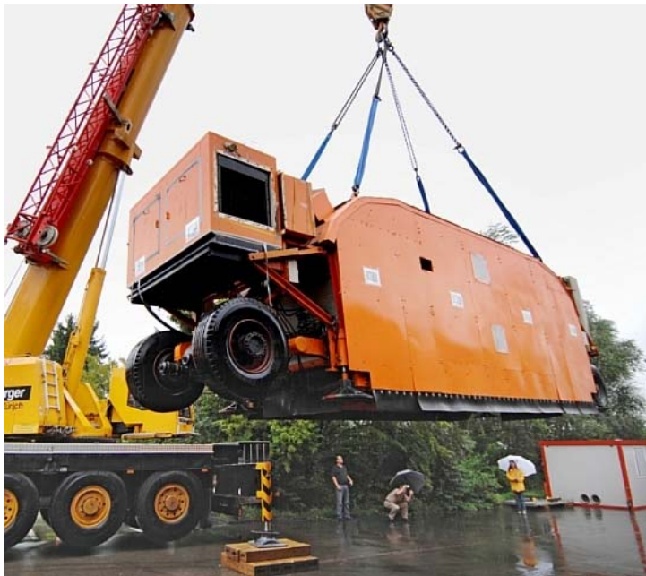
The mobile traffic load simulator «MLS10» from South Africa is unloaded at Empa
