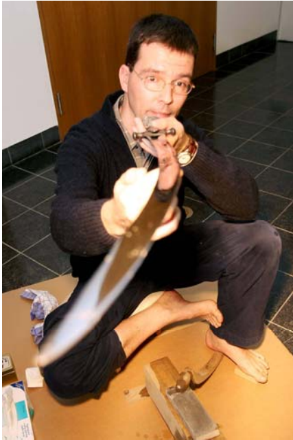
An alemannic blade from the 6 th century, from South Germany, after treatment by the kantei method. The bright area is the hardened steel in the blade; the darker area is softer, low carbon steel. (Photo: S. Maeder).
