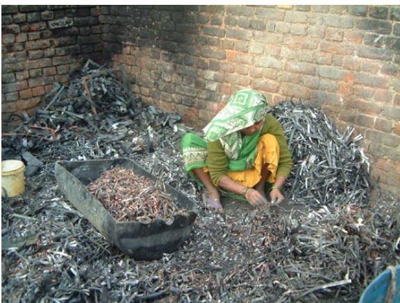
Indian woman segregating copper after burning printed circuit boards
