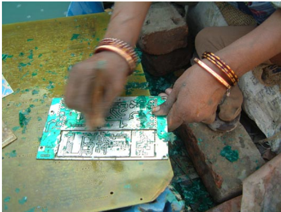
woman preparing printed circuit boards for copper leaching
