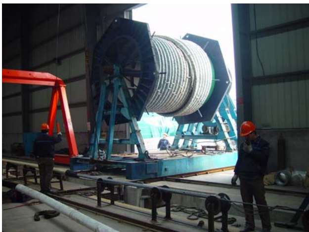
The 228 meter long bridge cable is transported to the test set-up.
