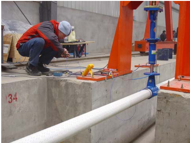
Measuring cable damping with feedback controlled MR damper.
