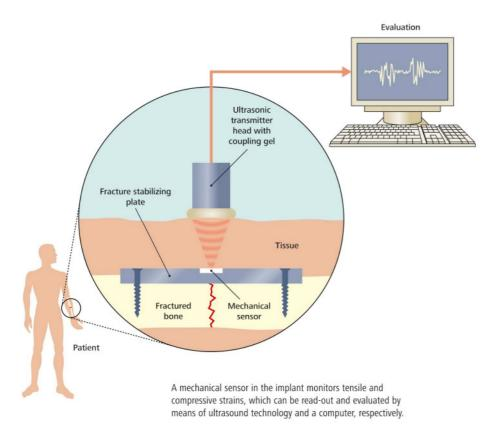
A mechanical sensor in the implant monitors the tensile and compressive forces it suffers. The measured data can be read out using an ultrasound device and analyzed by computer.
