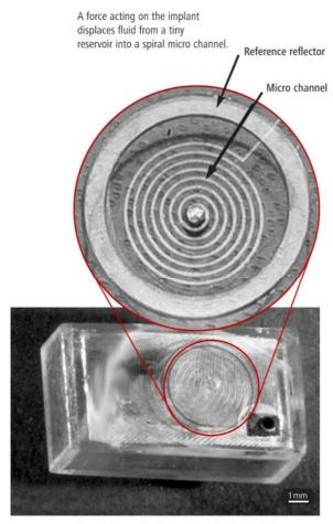
The passive mechanical sensor contains absolutely no electronics.
