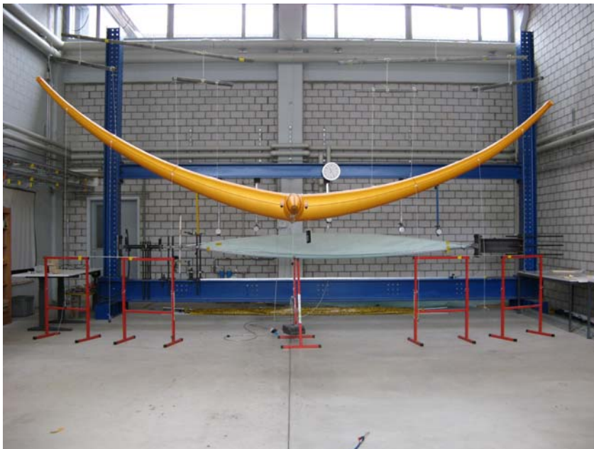
The Tensairity kite undergoing load tests in the laboratory.
