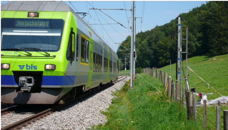
Noise emission measurements on a passing train. The measuring equipment is in the foreground to the right.
