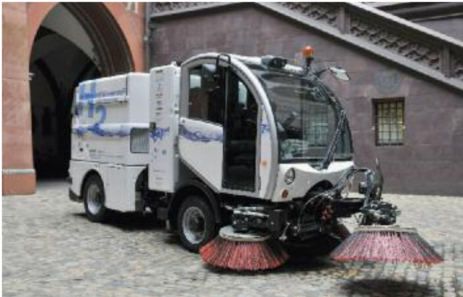
The “Bucher Schörling CityCat H 2 ” on the streets of Basel – in the first phase of this project, the world’s first municipal vehicle with a hydrogen powertrain consumes on average only half as much fuel as a conventional vehicle. (Photo: Juri Weiss)
