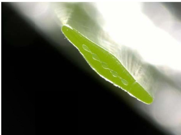
Cross-section of the fibre: It consists of five thin cores of polyamide and a sheath of polyethylene.
