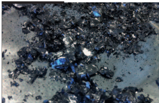
The result of a master's thesis: monocrystals with thermoelectric properties. (Photo: Empa)
