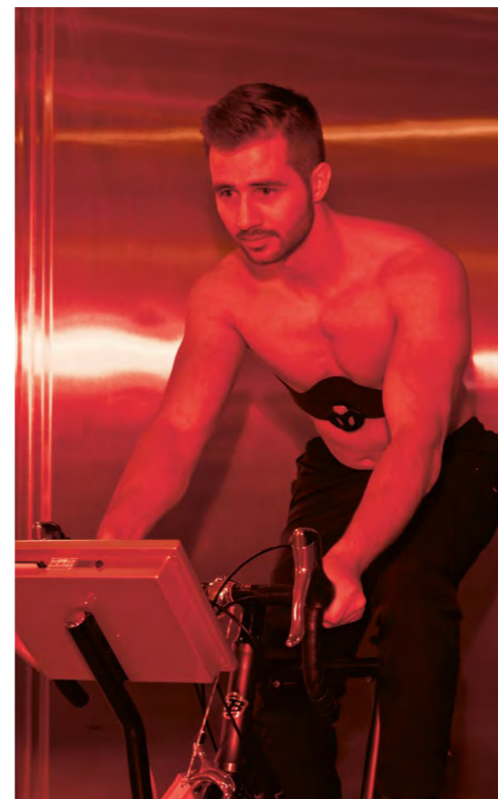
With the cardio belt made of comfortable fabric and embroidered electrodes, physiologically important parameters can be measured comfortably over a longer period of time. Image: Robert Stürmer / Empa
