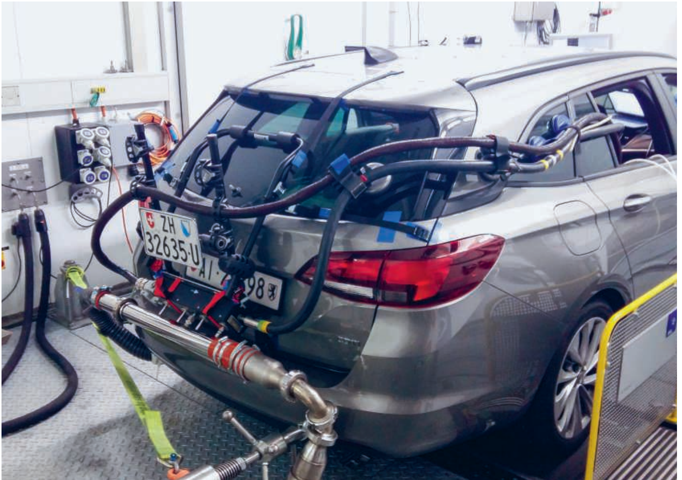
An Opel Astra 1.6 CDTI in the Empa exhaust laboratory. The pipes connect the exhaust system with a mobile PEMS (portable emission measuring system) in the inside of the car. After calibration of the measurement setup in the exhaust gas laboratory, it then goes onto the road.
