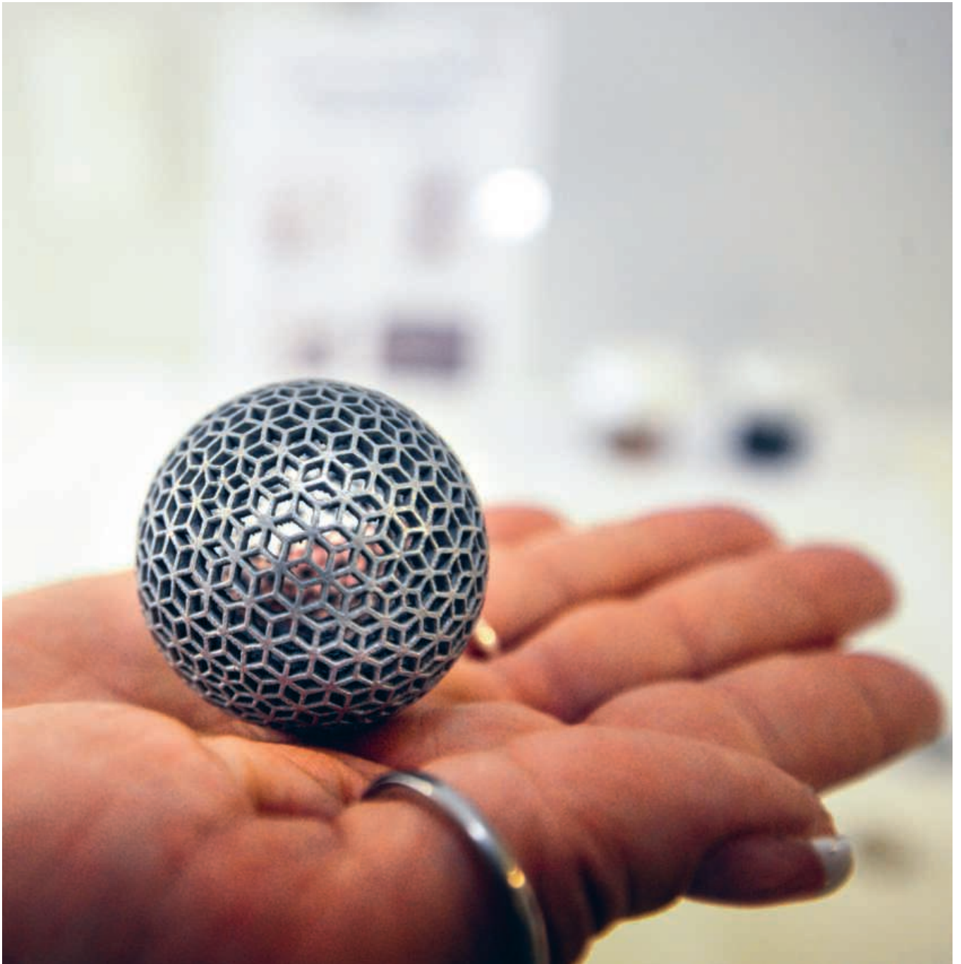
A lattice sphere made of an AlSi10Mg alloy, produced using the additive manufacturing method at ProtoShape GmbH, then irradiated and sanded. Design by George W. Hart.
