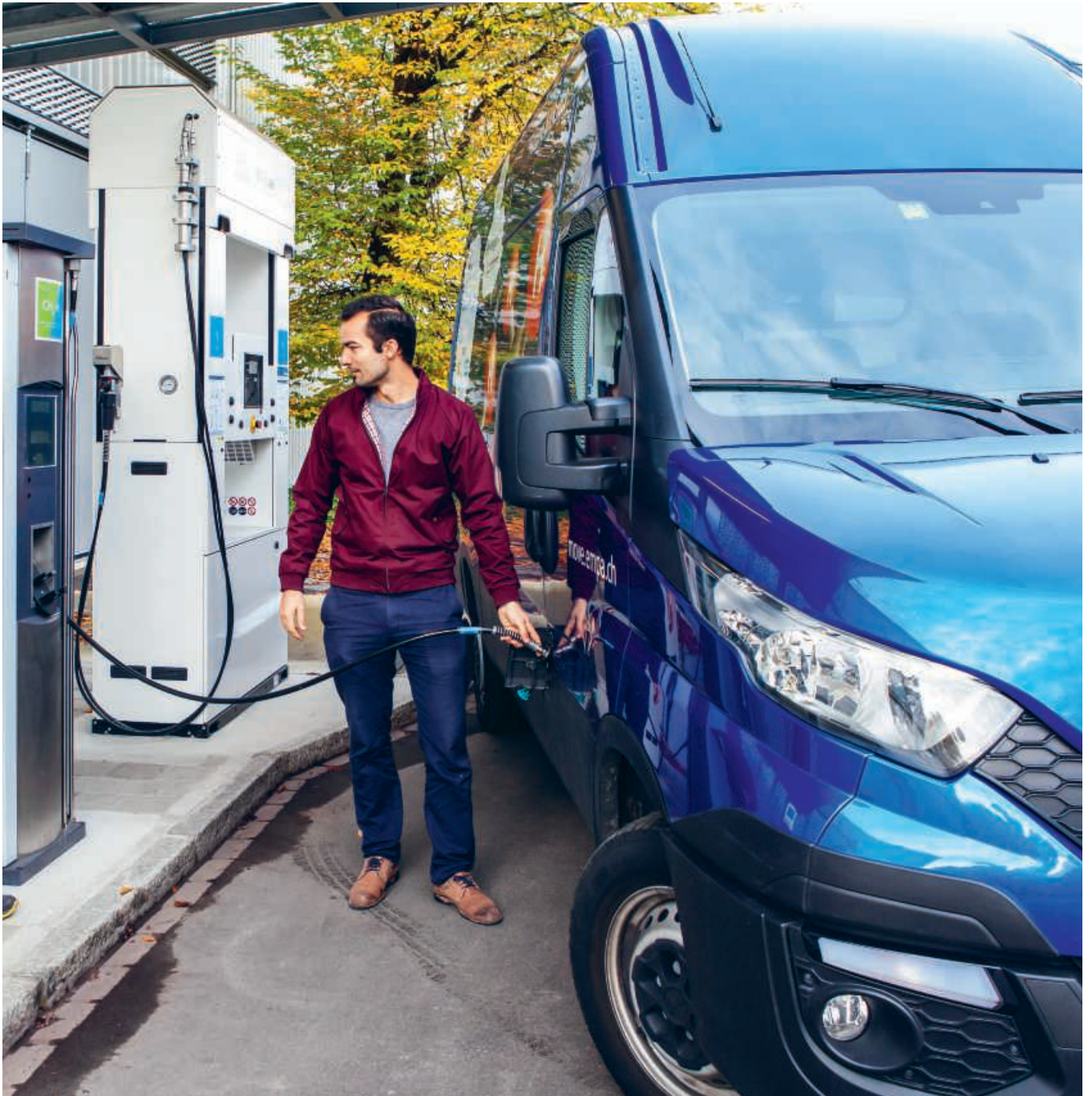
Swiss Post uses Empa's HCNG vehicle – here refueling on a mixture of methane and hydrogen – to deliver parcels since summer of 2017.
