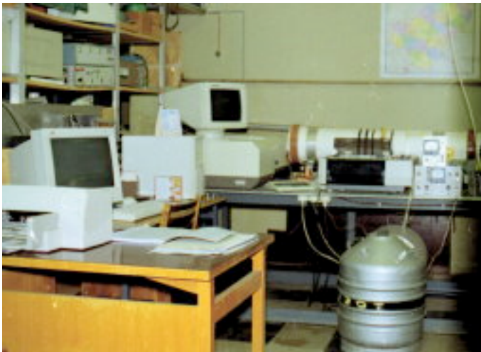
Figure 1 - Experimental setup with FTIR spectrometer and multipass cell (left) and new gas analyser MR-32 (right)
