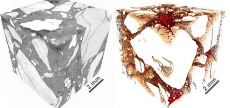
After every tomography the results will be processed and "volume segmentation" Finally, the segmented data from all
