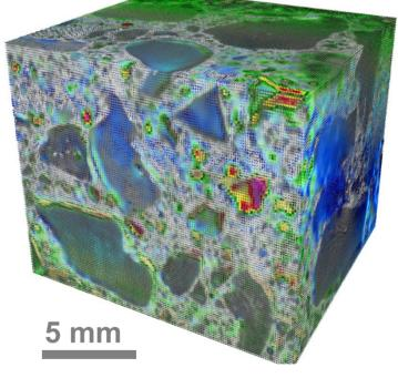
the ASR crack evolution (growth) in a one typical crosssections of concrete sample. The cross-sections are chosen from the volumetric (3D) temporal tomography data of exact same sample.
