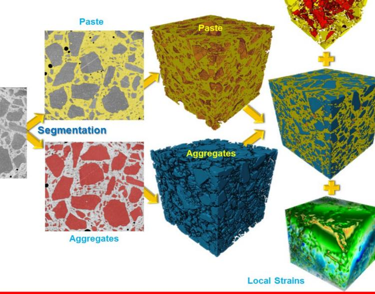
compared using "image registration" techniques and the strain amounts will be calculated quantitatively.
