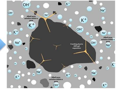
As a result of this reaction with an extremely hygroscopic product is formed. This product imbibes water existing in the pores and swells which is called as ASR gel. The gel expansion imposes stress into the concrete structure and instigates crack formation after exceeding the concrete tensile strength.
