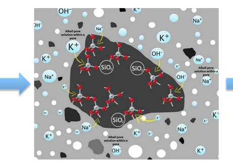
Alkali-silica reaction (ASR) is one of the most deleterious mechanisms in concrete structures since several decades [1-3]. Aggregate in within the concrete are surrounded by several pores filled with extremely alkaline pore solution. This pore solution can attack silicates within the aggregate and react.
