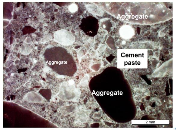
An example of optical microscopy (OM) image showing the general microstructure of the concrete samples. Aggregates are distributed within a homogenized cement paste.
