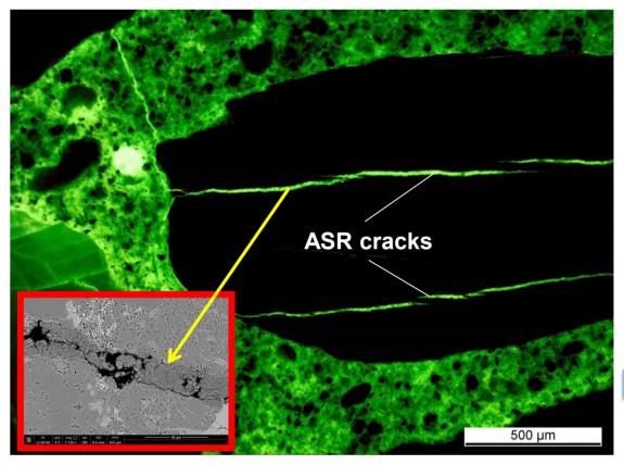
An example OM image showing the generation of ASR cracks in the expanded concrete structure. The ASR cracks are obvious within the aggregates and they have run into the cement paste.
