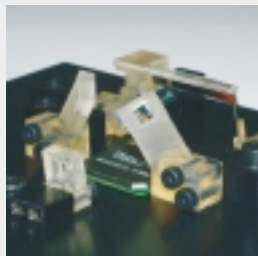
Fig. 5 Implementation of the illumination system
