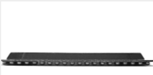
Fig.1 Ball Grid Array (BGA) viewed from the side.
