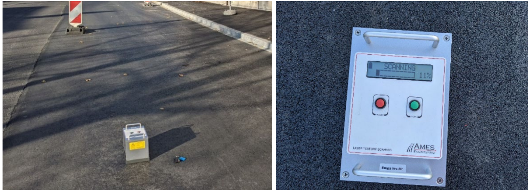
Fig. 50 Surface texture measurement device
