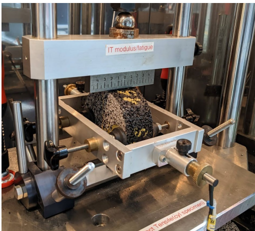
Fig. 42 Stiffness modulus and fatigue test setup
