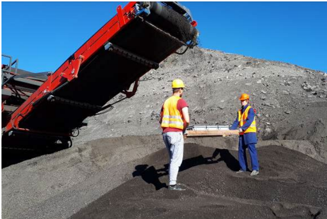
Fig. 55 Sampling of processed RAP directly from the belt to minimize variability
