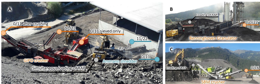
Fig. 52 The four crushers during the experiment (A - GIPO and Ammann, B - Benninghoven, C - SBM)
