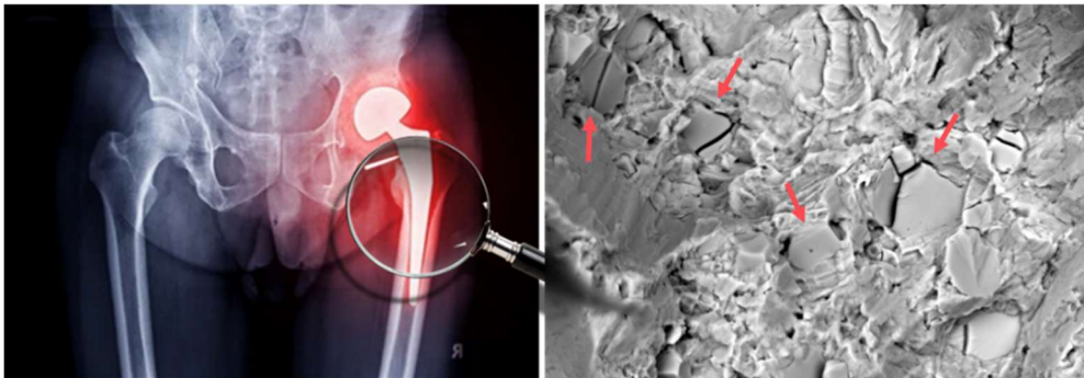
Fig. 1: left: X-ray showing a total-hip replacement, one of the clinical use cases of Co-Cr-Mo alloys; right: SEM image of the alloy with marked carbides contained in the microstructure (red arrows)
