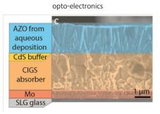
The aqueous solution deposition of transparent (> 90% transparency in visible light) and conductive (5 x 10<sup>-3</sup>  $\Omega$ cm) AZO films can be applied to diverse optical and opto-electronical applications such as e.g.:
