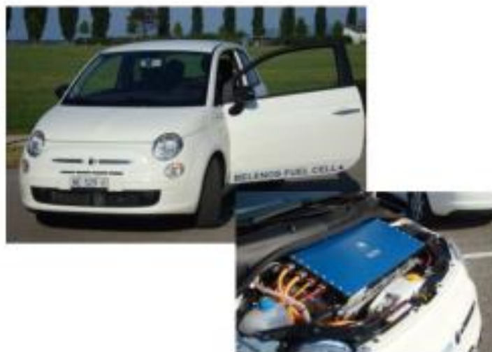
2013, Belenos develops the H 2 /air fuel cell systems and integrates it into a Fiat 500
