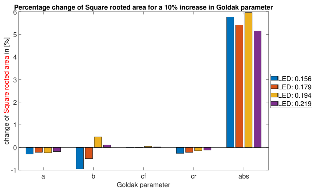
Figure 3.7.: Change of the melt pool square rooted area shown in percent for a 10% change in each Goldak parameter while the other parameters are kept constant.
