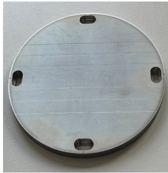
Figure 2.1.: Main plate for the LPBF process made of Hastelloy X.
