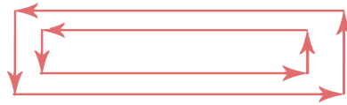
Figure 2.7: The scan strategy used for thin walls consisted of two rectangular contours. The outer ones were printed at once before the inner ones for all structures.
