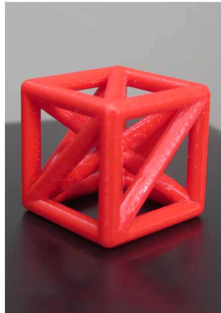
Figure 4.1: Unit cell model of the lattices manufactured with fused deposition modeling (FDM)
