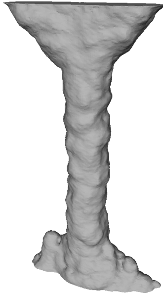
Figure 2.11: \mu -CT scan converted to STL-file of an AM Ti-6Al-4V strut with 200\mu\text{m} nominal diameter (strut S1_4_1 ).
