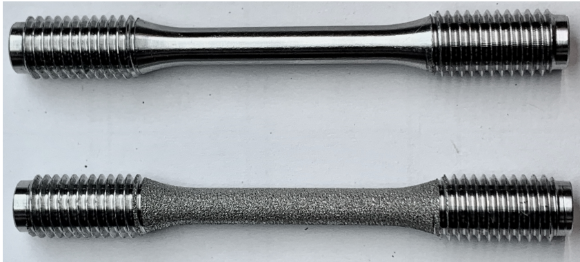
Figure 3.2: Comparison of the two versions of the specimen used for mechanical testing. Top: surface machined, bottom: as-built.
