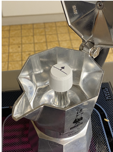
Figure 4.4: Experimental Verification of Splash Guard Concept
