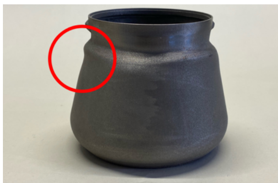
Figure 6.1: Buckling Visible in Boiler Print
