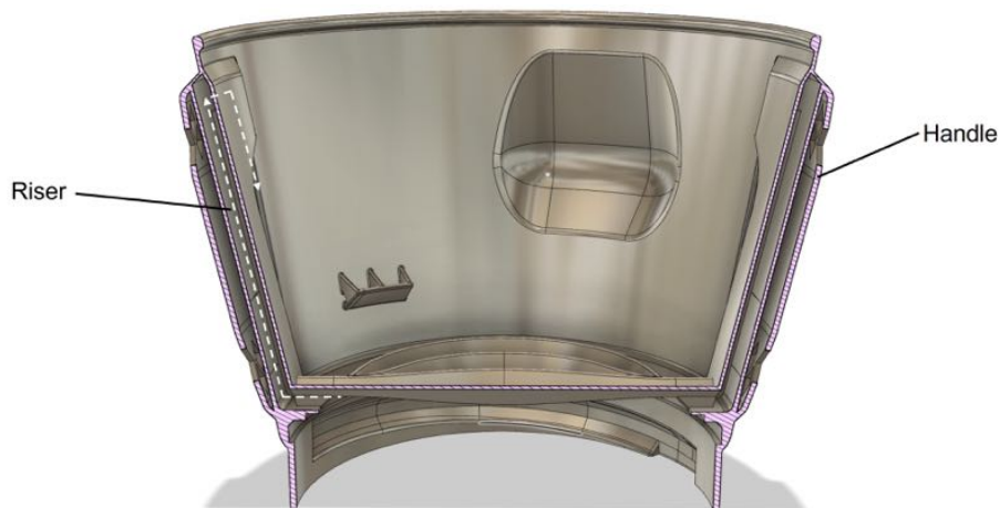
Figure 5.9: Cross Sectional View of the Cup
