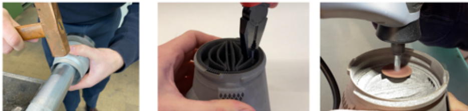
Figure 6.5: The Three Manual Post Processing Steps: "Unwarping", Support Removal and Grinding
