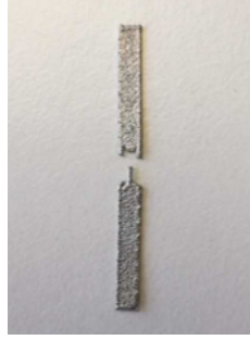
Figure 3.7: Picture of a strut specimen that failed at the transition region.
