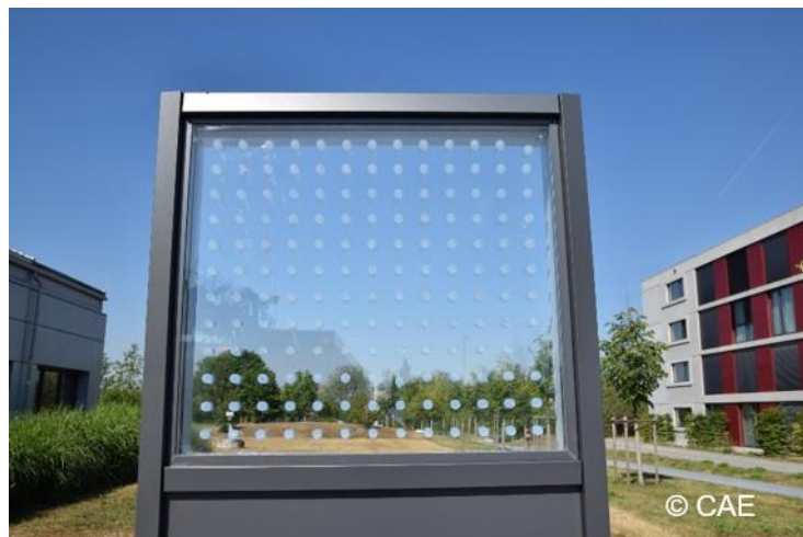
Fig 1. Demonstrator of vacuum glazing with transparent silica aerogel pillars.
