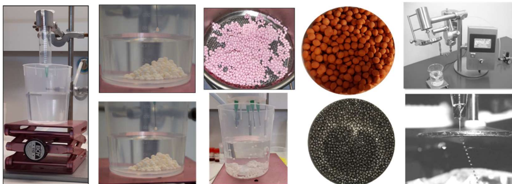
Fig. 1. Overview of the RF and Carbon Aerogel Micro-beads Production.
