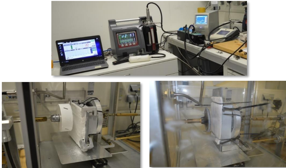
Fig 1. Cutting using a circular saw and sanding, inside a particle-free chamber. Aerosol release monitored in parallel by Optical particle sizer (OPS), Condensation particle counter (CPC) and Electrical low pressure impactor (ELPI)
