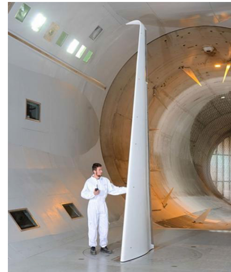
ONERA- natural laminar flow test of a semi span wing at an ONERA wind tunnel
