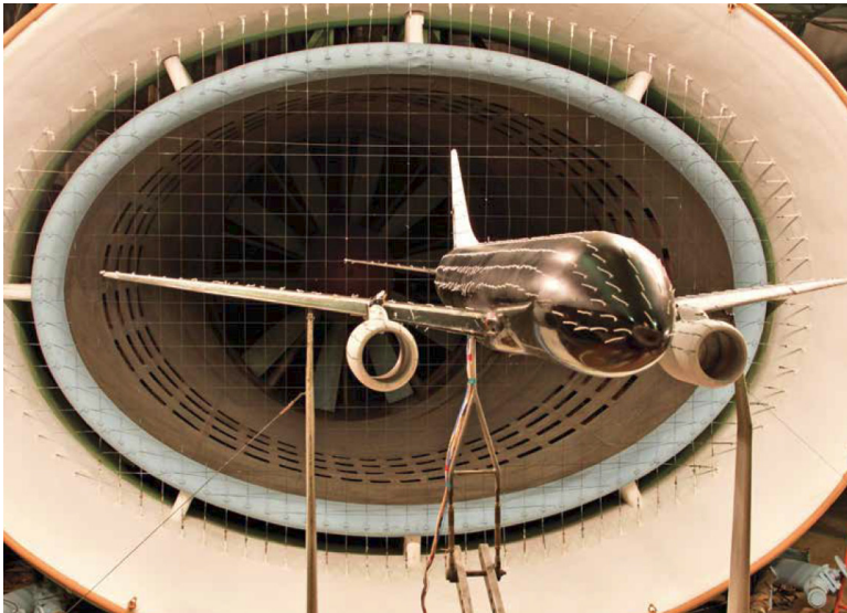
T-103 full a/c wind tunnel testing in Tsagi
