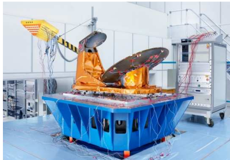
Figure 2.1: Full CFRP antenna reflector, partly covered with MLI
