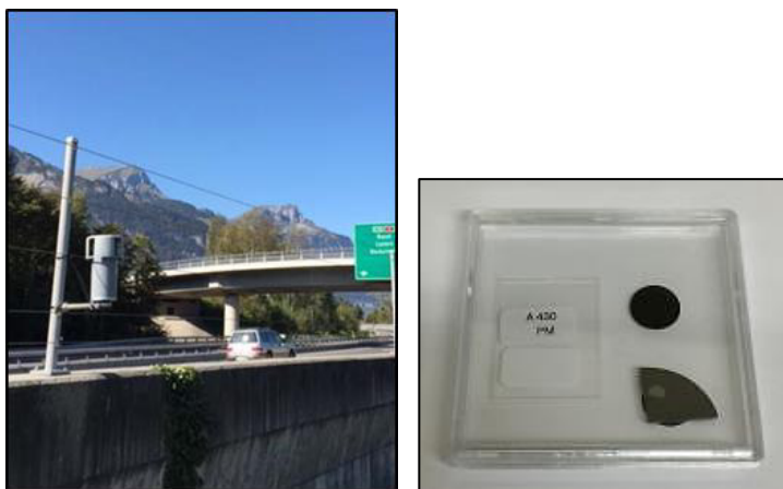
Figure 1: Left image: Sigma-2 passive sampler; right image: adhesive surface with different substrates. Boron (lower right corner) and carbon pad (upper right corner) for REM/EDS analysis. Glass plate (left) for light microscopy.
