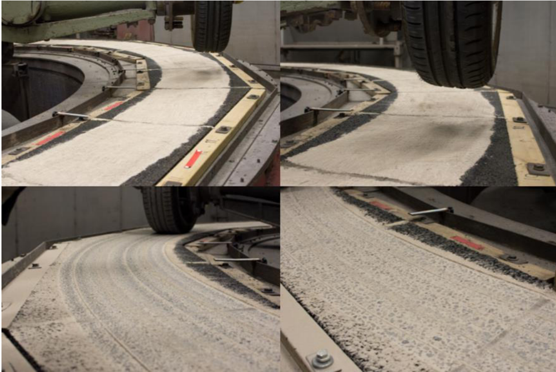
Figure 4: Road surface after application of dust (top figures) and after 1200 tyre passages with residual dust left in the road surface texture (bottom figures).
