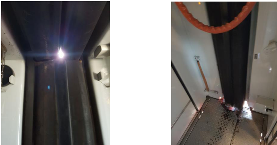
Figure 5: Ruptures in rubber connectors between the carriages.
