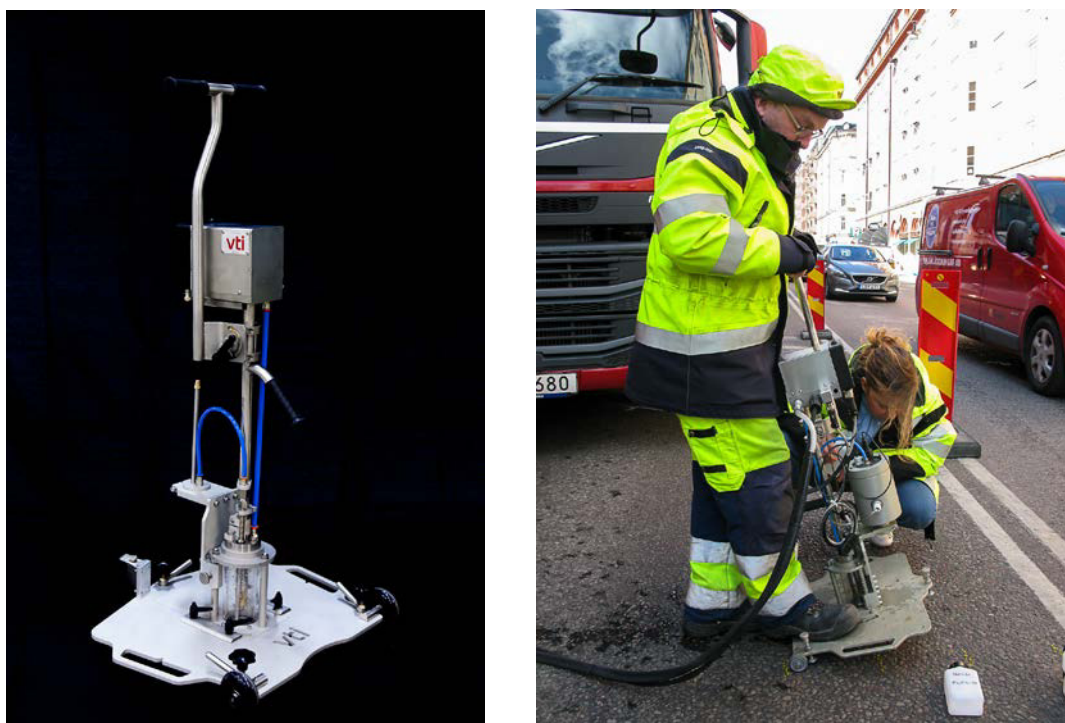
Figure 1. The wet dust sampler (WDS) in the laboratory (left) and in the field (right). (Photo: Mats Gustafsson, VTI).
