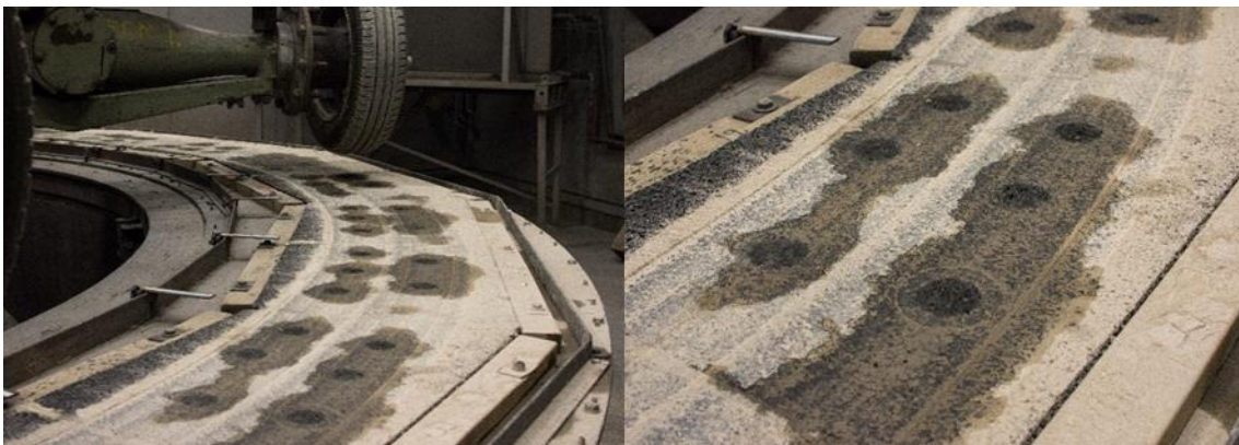
Figure 5: Example on road surface after WDS sampling. In the right figure, 6 samplings were performed, divided into 5 sampling stored in a large bottle and 1 sampling stored in a small bottle.
