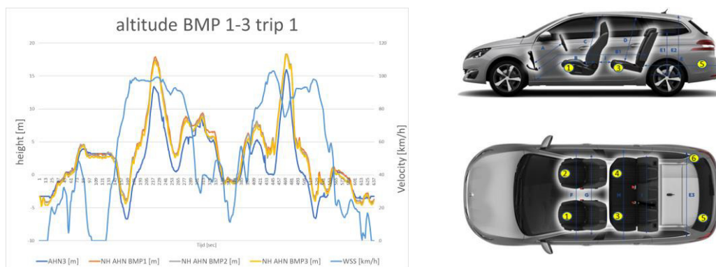
Figure 3 Different pressure sensors (BMP1-3) in the vehicle compared with the map-based altitude (AHN3). With the higher velocities, all sensors show a systematic deviation upward of a few metres, associated with a lower pressure readings.
