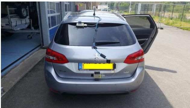
Figure 7 The vehicle with SEMS equipment in and under the car and different pressure sensors installed at the back can be operated in normal use.
